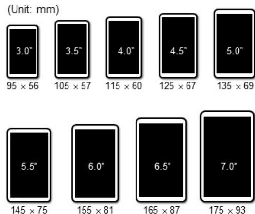
Figure 1. Nine different sizes of smartphone mock-ups
