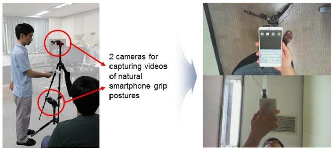
Figure 2. Smartphone grip posture measurement environment
