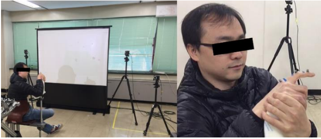
Figure 2. Experimental setting with five infrared cameras for capturing hand motion and a chair with an arm supporter to fix the forearm and hand.
