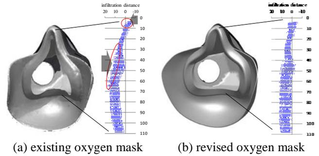
Figure 3. Fit analysis for the existing and revised oxygen mask
