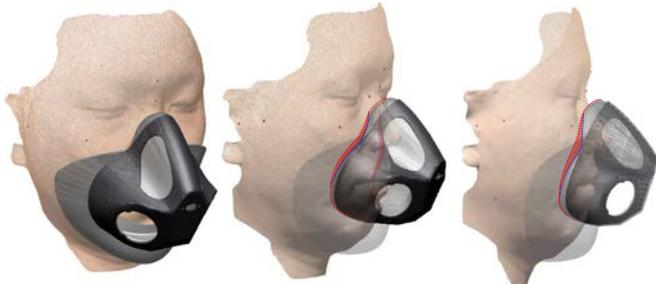
Figure 1. Illustration of a virtual fit analysis of an oxygen mask design on a pilot's face
