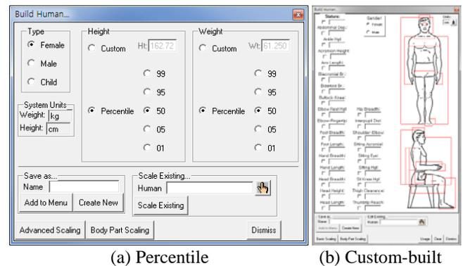
Figure 1. An example of RHM generation interfaces of Jack<sup>®</sup>
