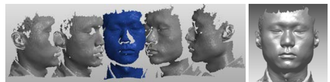
Figure 3. Initially 3D scanned images (left) and the post-processed image (right)
