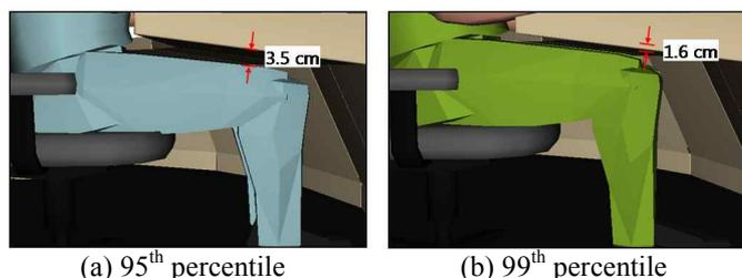
Figure 5. Clearance of the console for operator’s upper leg
