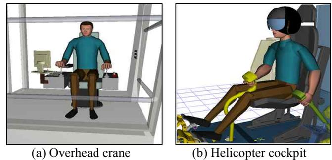
Figure 1. Ergonomic evaluation using digital human simulation
