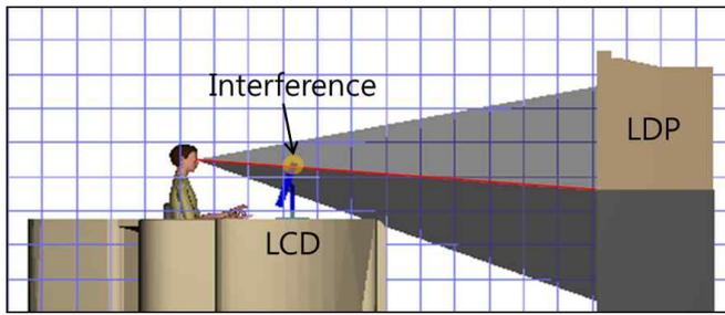
Figure 8. Vertical gaze interference between LCD and LDP
