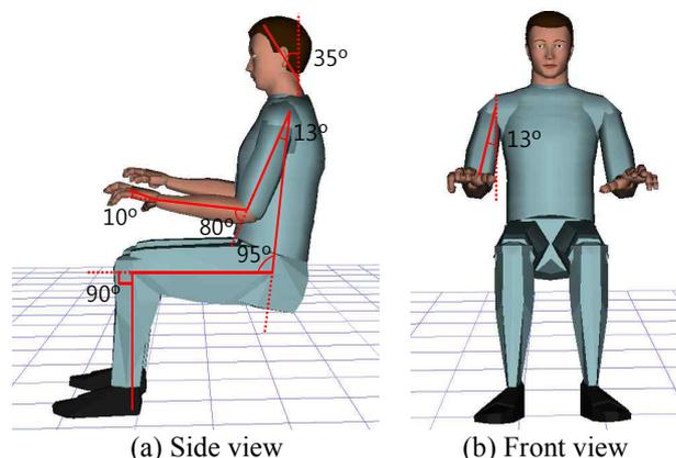
Figure 4. Reference posture of operators in the MCR
