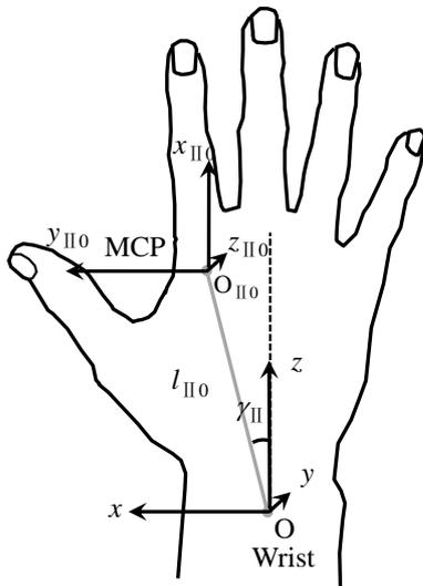
Figure 3. Relationship between the global coordinate system and the local coordinate system of the index finger
