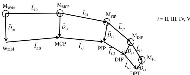
Figure 4. Geometric relationship between surface markers and internal joint centers
