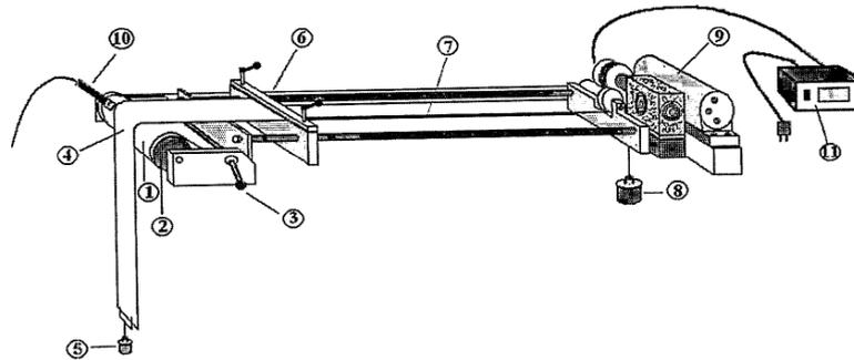
**Figure 3. Diagram of MAFN: (1) Fabric, (2) stationary pully, (3) closing lever, (4) fabric 2, (5) load (0.5kg), (6) movable rope, (8) load (9) door closer, (10) microphone, (11) speed meter**
