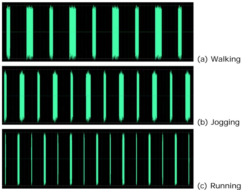
Figure 6. Simulation of fabric sound according to wearer's activities
