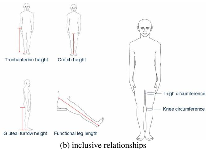
Figure 3. Types of geometric relationships between anthropometric variables (illustrated)
