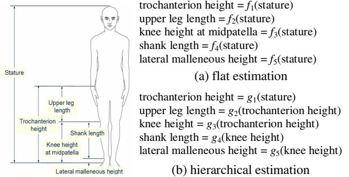
Figure 1. Comparison of flat and hierarchical estimation methods.
